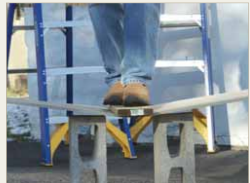
When compared to Structure® EPS, common vinyl siding panels fold under the pressure.
